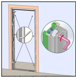
3.Adjust the frame to fit the wall opening properly by tightening the 6 anchors (attached to the frame) with a 12mm Allen Wrench (not provided).
