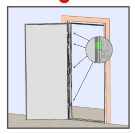
6.Install the door slab onto the frame with the hinge plates. Make sure to align the slab with the frame properly to allow door opening and closing freely.
