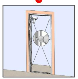
4.Drill a hole in the wall through the center of the hexagonal adjustable bolt to install the fixing screw. (If using our accessory B, handheld electric drill and 10mm drill bit are required for drilling)
