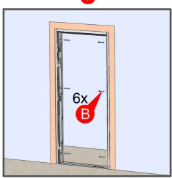
5.Choose a proper wall-screws (B) based on your wall material type: B-1 or B-2, Place your chosen 6pcs wall-screws to each anchor and tighten them as shown in image.
